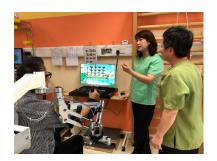
Armeo Spring system is an instrumented arm orthosis with a spring mechanism for enhancing upper extremities function. It produces adjustable sensitivity of grip strength sensing, thus achieving the augmented feedback that promotes functional training.
